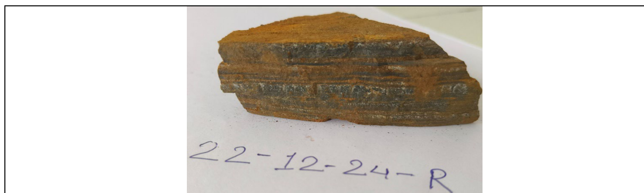
Figure-40: Photographs of the hand specimen showing dark to light grey coloured nature of the rock.
