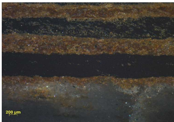
Figure-43: Alternate bands showing subangular Quartz embedded within iron oxide (Magnetite) minerals .
