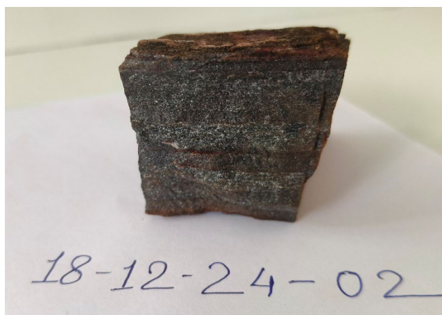
Figure-34: Photographs of the hand specimen showing dark to light grey coloured nature of the rock.
